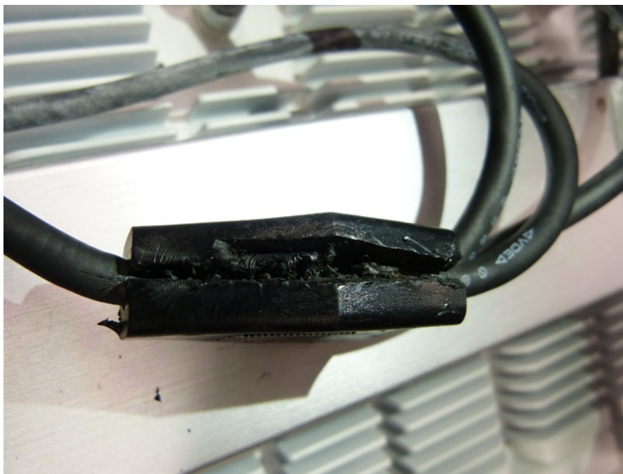
View of wire distributor after IPX7 test
