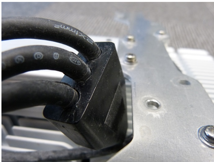
View of wire distributor after IPX7 test
