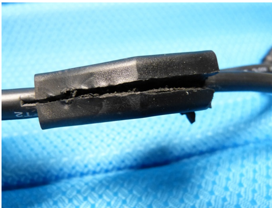
View of wire distributor after IPX6 test
