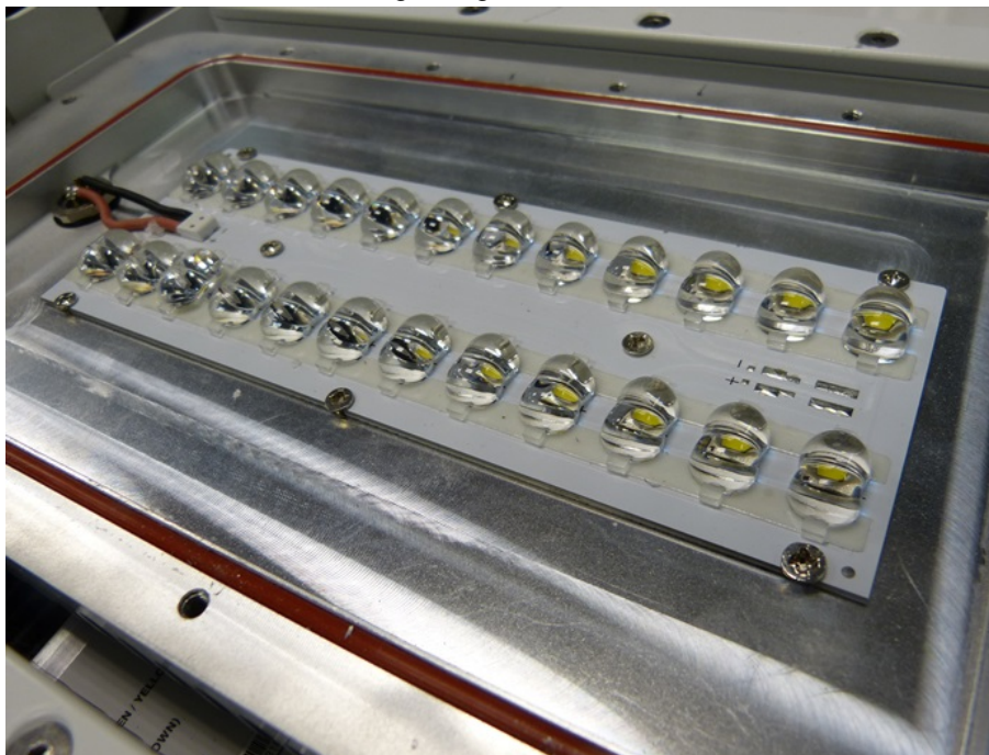
View of light engine after IPX6 test
